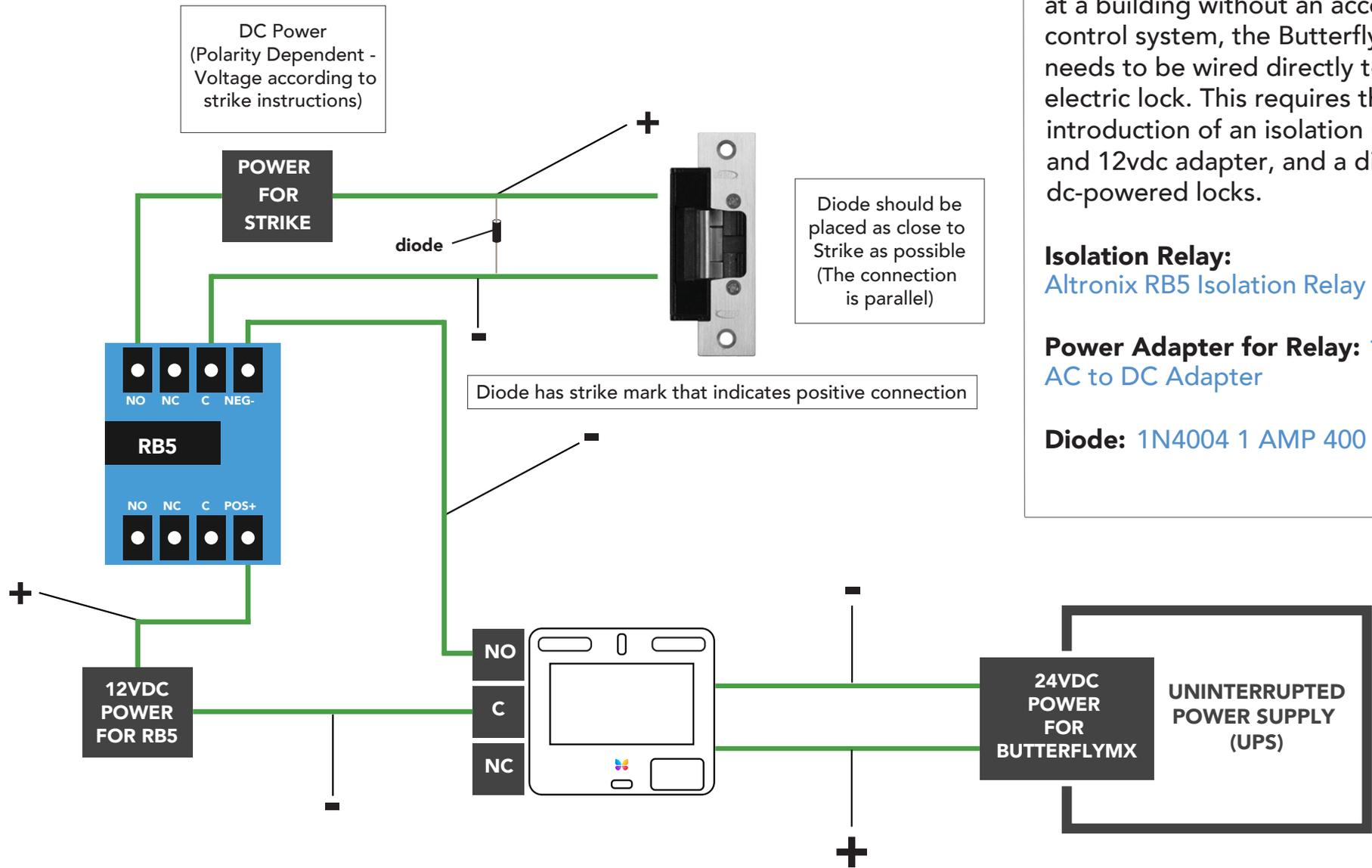
When installing a ButterflyMX panel at a building without an access control system, the ButterflyMX needs to be wired directly to an electric lock. This requires the introduction of an isolation relay and 12vdc adapter, and a diode for dc-powered locks.
